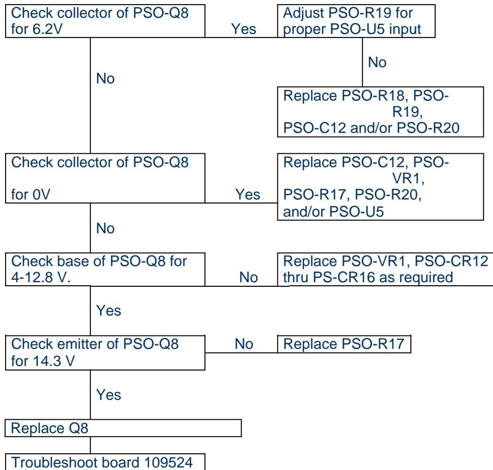
Figure 105. Fault #1 Diagram (4 of 4)
