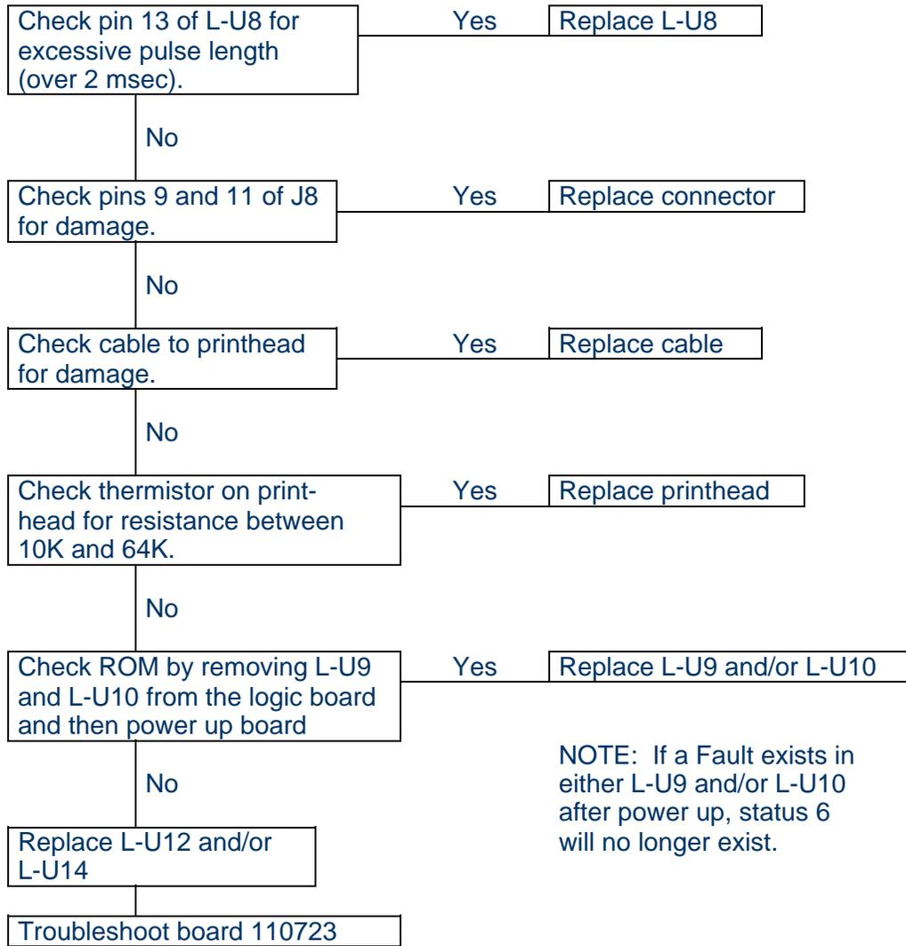
Figure 106. Fault #2 Diagram (2 of 2)
