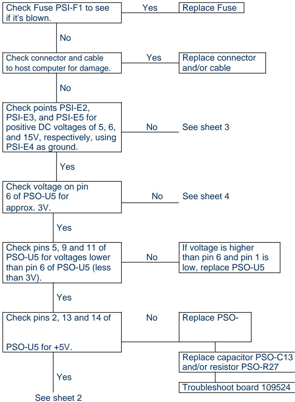
Figure 105. Fault #1 Diagram (1 of 4)
