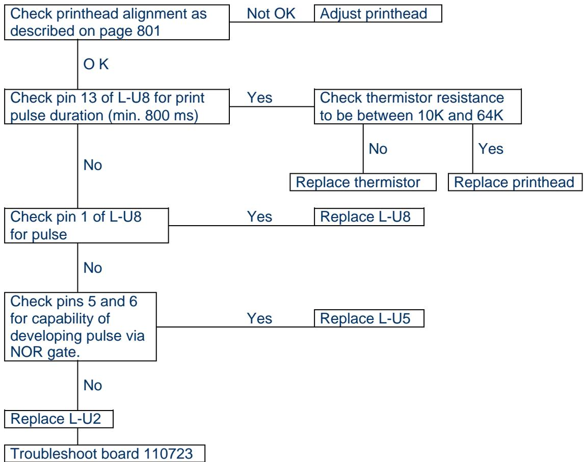
Figure 112. Fault #8 and #9 Diagram
