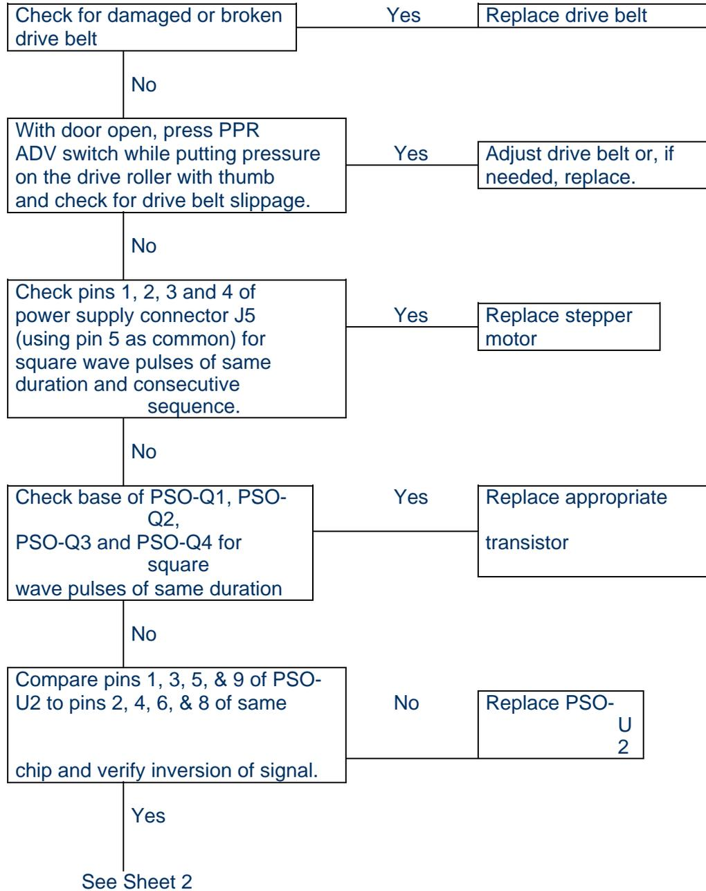
Figure 107. Fault #3 Diagram
