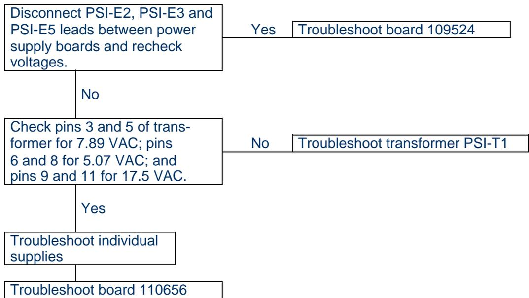
Figure 105. Fault #1 Diagram (3 of 4)
