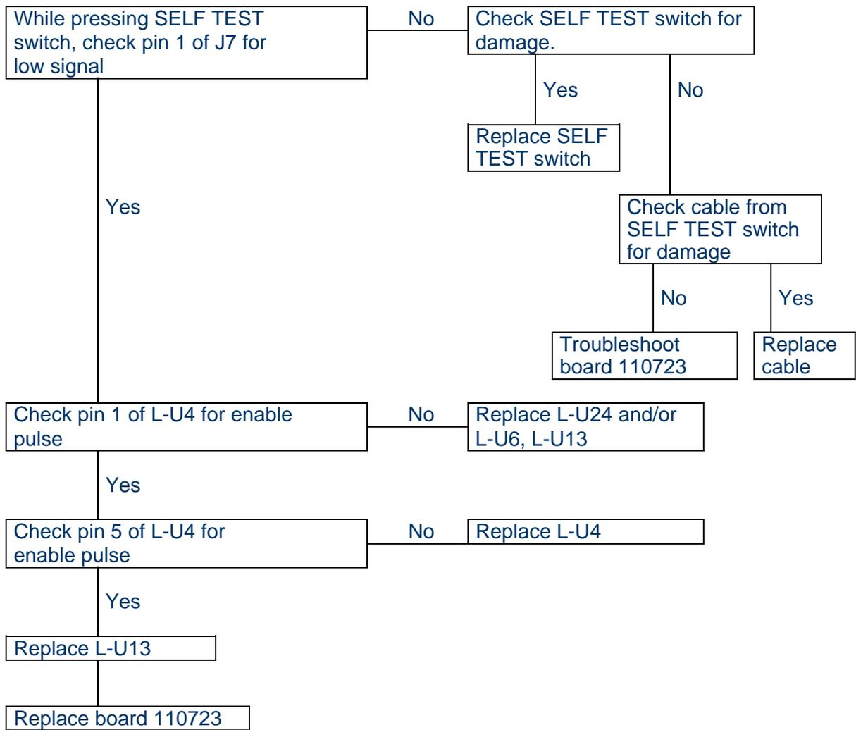
Figure 109. Fault #5 Diagram
