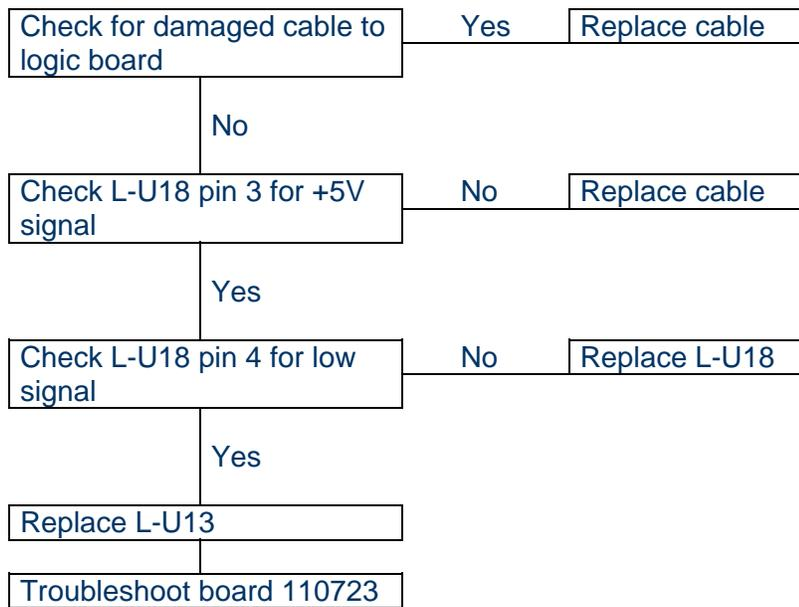
Figure 105. Fault #1 Diagram (2 of 4)
