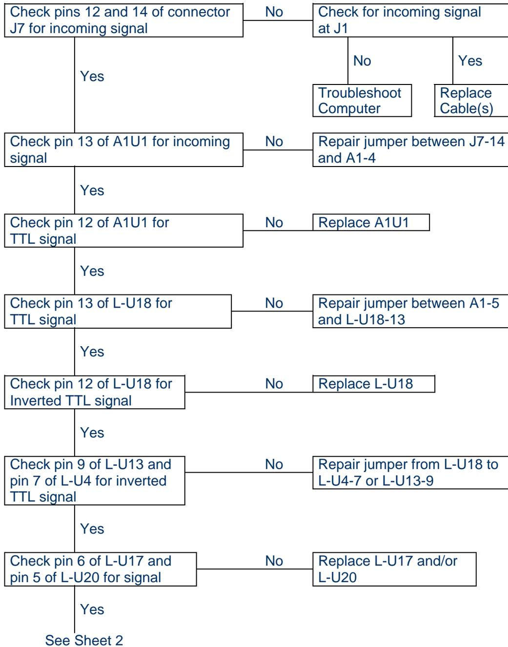
Figure 108. Fault #4 Diagram (1 of 2)
