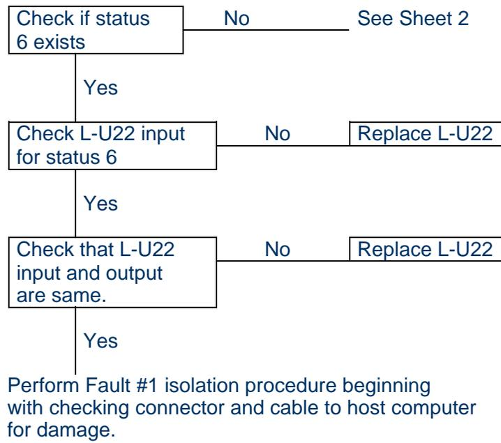
Figure 106. Fault #2 Diagram (1 of 2)
