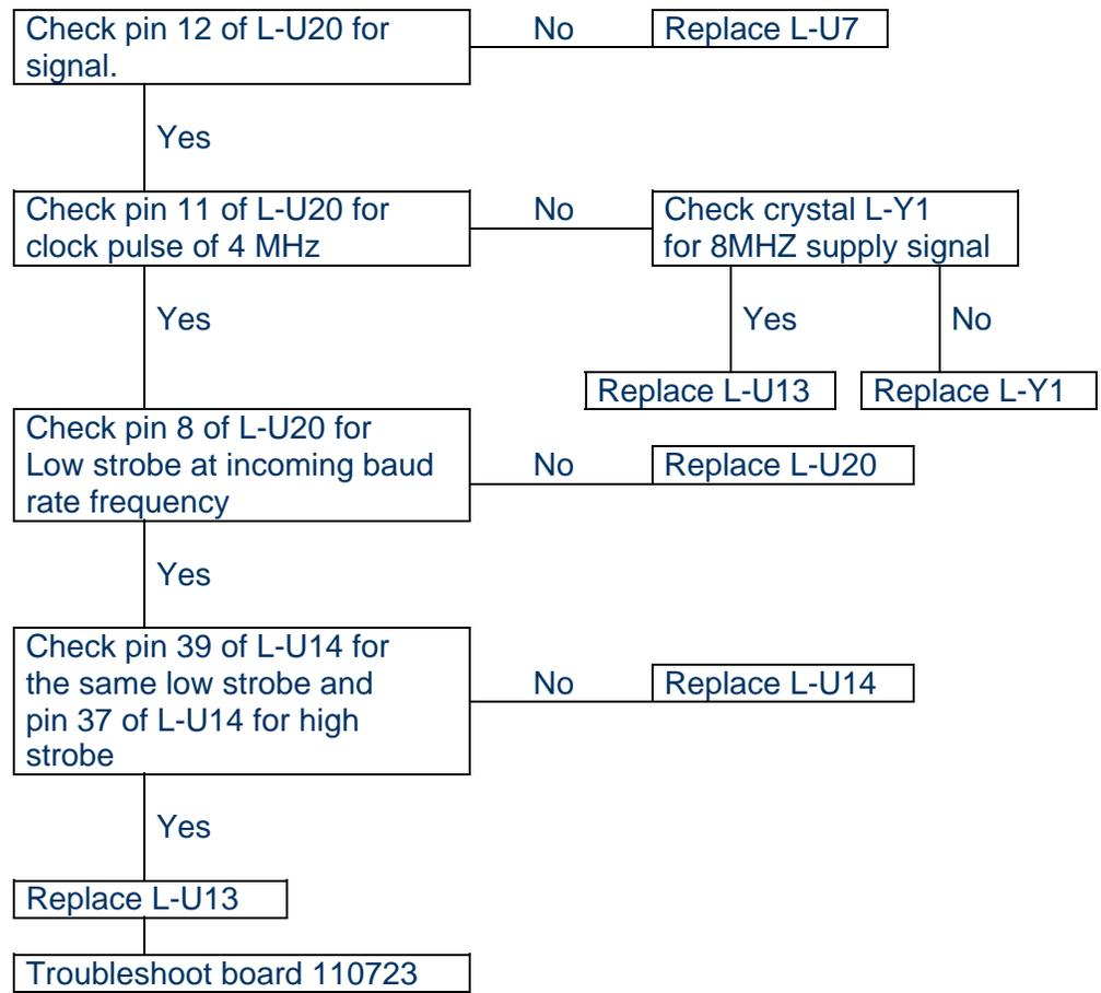
Figure 108. Fault #4 Diagram (2 of 2)
